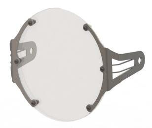
Assemble polycarbonate lens to stainless frames. Peel protective film back from polycarbonate lenses. Use T10 torx and 5.5mm nut driver to attach lenses to frames. Place M3 torx screws and washer against polycarbonate, and with M3 locknut on back side agains stainless steel frame.
