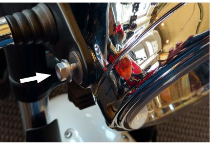
Use 12mm socket to loosen one of the hex screws that holds the headlamp in place. Do not remove all the way. (TIP! this will be easier if you have a friend to help hold the headlamp in place).
